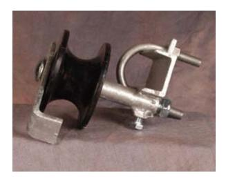
The FS-2000br slide gate track roller is made of injection molded Deleron for high durability. This model can be ordered with or without mounting bracket
